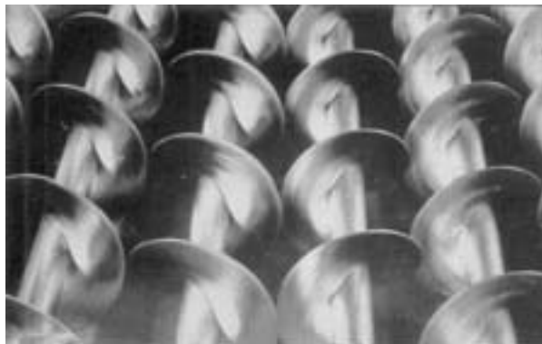
Figure 21 Wear on meat grinding equipment is greatly reduced by electroless nickel.
