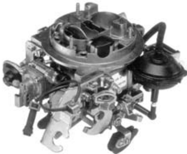
Figure 28 Electroless nickel resolved corrosion problems on carburetors using ethanol fuel.
