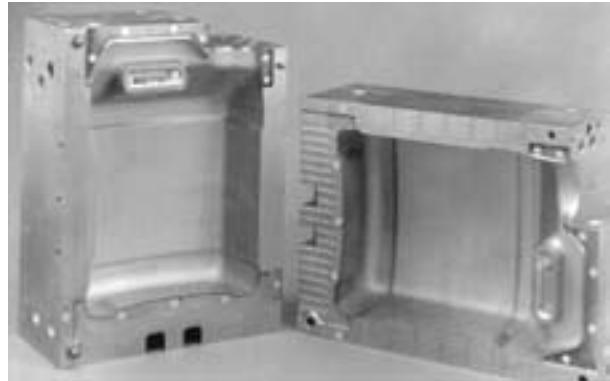
Figure 43 Electroless nickel prevents wear and corrosion of aluminum blow molds.
